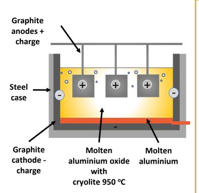
Aluminium oxide has a very **high melting point** so is mixed with molten **cryolite** to lower the temperature required to carry out the electrolysis. Aluminium goes to the negative electrode and sinks to bottom.
