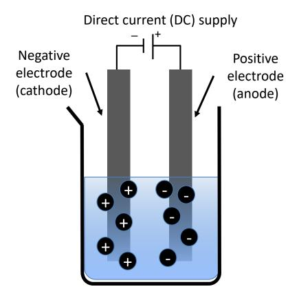
**Positive** ions go to **negative** electrode (cathode) and are **reduced** (gain of electrons).
