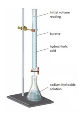
2. Fill the burette with acid and note the starting volume. Slowly add the acid from the burette to the alkali in the conical flask, swirling to mix.
