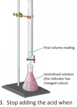
3. Stop adding the acid when the end-point is reached (the appropriate colour change in the indicator happens). Note the final volume reading. Repeat steps 1 to 3 until you get consistent readings.
