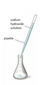
Use the pipette to add 25 cm<sup>3</sup> of alkali to a conical flask and add a few drops of indicator.
