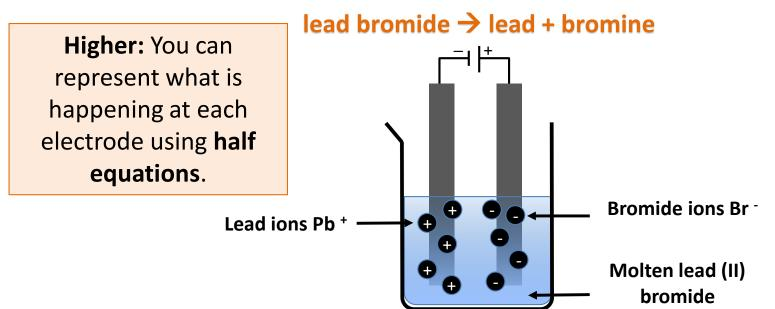
The positively charged lead ions Pb + (cations) are attracted to cathode and the negatively charged bromide ions Br - are attracted to the anode.
