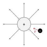
Draw the pattern of electric field lines in the space around the positivelycharged collecting sphere.
