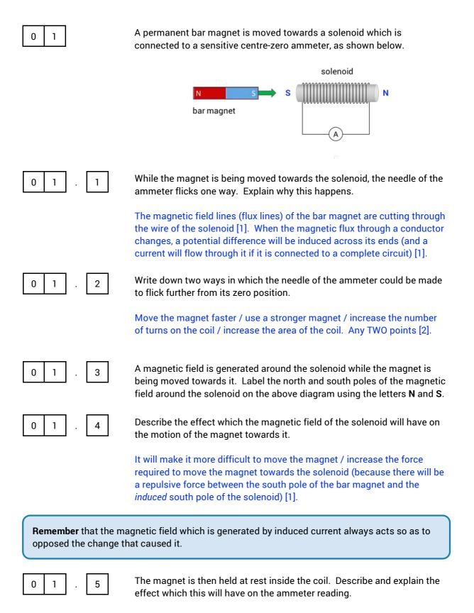
The ammeter reading will fall to zero [1] because the magnetic flux through the solenoid will no longer be changing / the rate of change of magnetic flux through the solenoid will fall to zero [1].
