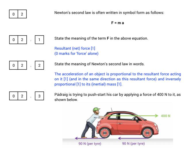
If the force of friction acting between **each tyre** and the road is 90 N and the mass of the car is 1600 kg, calculate its acceleration. You may neglect the effects of air resistance in answering this question.
