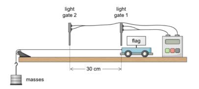
The light gates are set up so as to measure the average velocity at which the trolley is moving as it passes through them.
